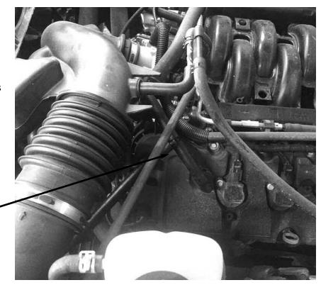
The drain hose can be routed out the bottom of the truck to make for easier draining of the main catch can. Generally draining every oil change is sufficient but each application is different. Do not let the can fill with oil / vapor fluid as it could cause engine damage. Draining more often in cold climates is required so the fluid does not freeze in the can.
