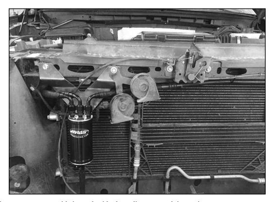
Route the two passengers side hoses beside the radiator toward the engine. Screw hoses to the catch can as shown on the hose labels.
