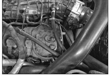
Install the small CSS can (Clean Side Separator) using stock bolt on drivers side firewall by the brake booster.
