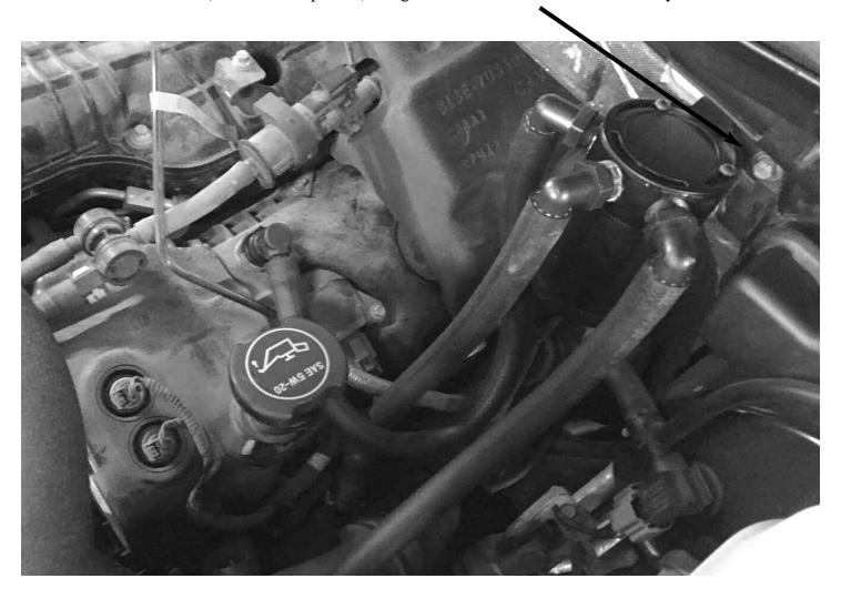
Remove the stock PCV tube that runs from valve cover to turbo inlet tube.
