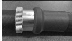
Use shrink wrap to secure the check valve into hose. Be sure arrow is pointing toward engine and cover both hoses with shrink wrap.
