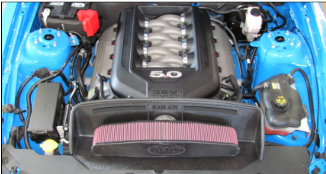
The finished install showing front mounted filter, ram air box and relocated coolant tank
