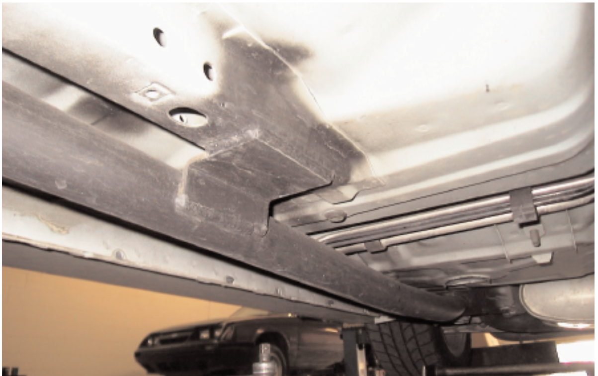
Picture 2 - View from middle to rear of subframe connector showing middle bracket welded to front subframe and rear bracket welded to the rear bulkhead.
