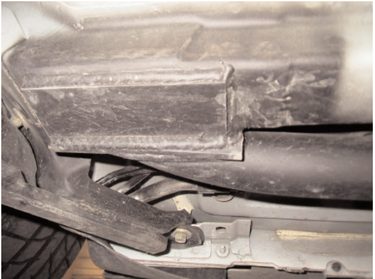
Picture 3 - Detail of front bracket and connector welded to front subframe.
