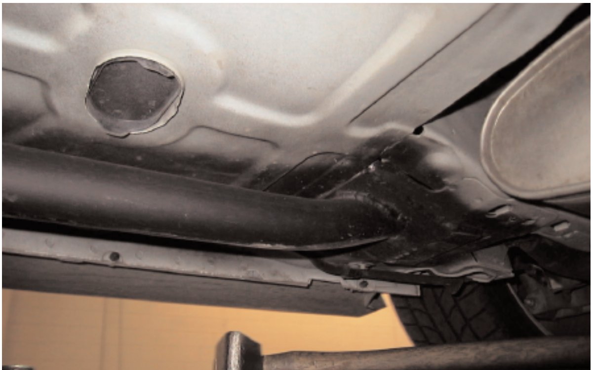
Picture 4 - Detail of rear connector and bracket welded to rear bulkhead on 94-04 Mustang.
