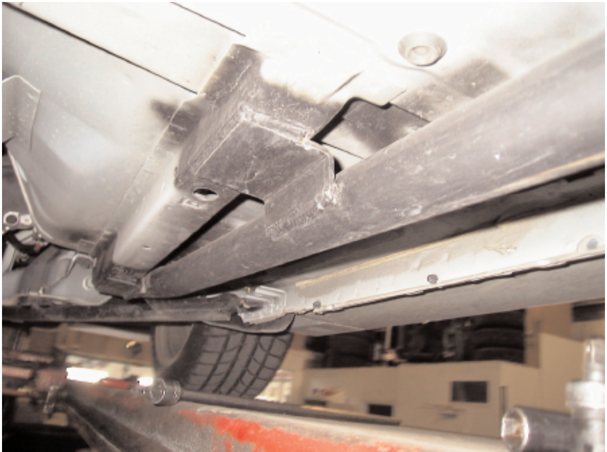
Picture 1 - View from middle to front of subframe connector showing middle and front brackets welded to the front subframe.
