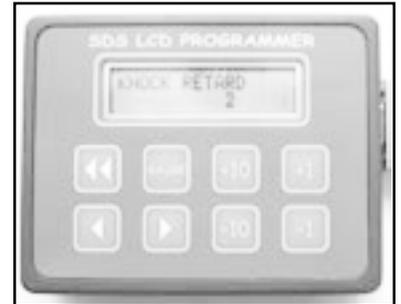
If you wish to turn off the knock sensing option, you can enter a 0 in the KNOCK RETARD parameter. The knock sensing option can take the place of large amounts of MAP retard in some cases, however, total reliance on the sensor while running unrealistically high amounts of spark timing may lead to running problems. We recommend using the knock sensor as a safety device rather than a primary timing control.
