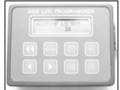
If changing the values will not make the engine respond properly, check to make sure that the TPS is hooked up correctly. You can check for proper operation by selecting GAUGE 2 mode. You should see the AP number increase from 0 to a higher number when the throttle is rapidly opened, then as the throttle movement stops, the number should quickly return to 0. The AP number should always be 0 when the throttle is not moving. If not, it indicates an intermittent connection or a damaged TPS.
