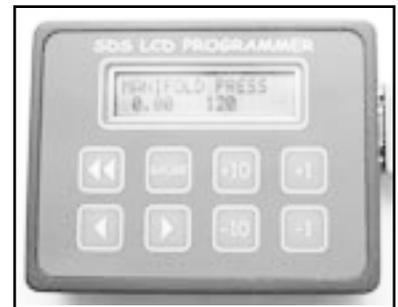
All units are pre-programmed with a standard MAP program, depending if the system is 1, 2 or 3 bar. These values should be close, so most **initial programming should be done on the RPM FUEL values**. If the engine appears to be too rich everywhere, lower the RPM FUEL values across the board. Do not start re-programming the MAP values as this often leads to people getting way off track.
