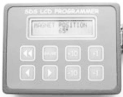
The MAGNET POSITION function on the SDS Programmer. Use the +1 and -1 buttons to adjust the value as described above.
