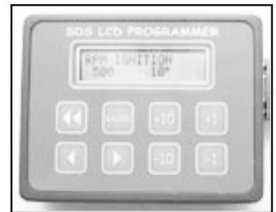
**It is critical that the RPM / IGN value at 500 rpm matches base timing set on your balancer. In the table above that would mean base timing at the balancer must be 10 degrees BTDC.**
