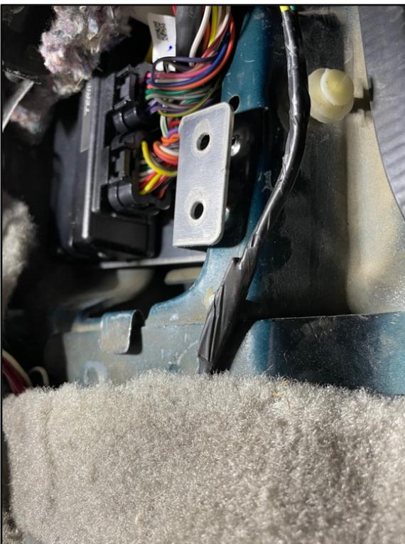
Earlier Fox Mustangs do not have the same opening for the ECU. Modifications to the bracket are required for mounting. Max ECUs for automatics will require the bracket mounted lower.
