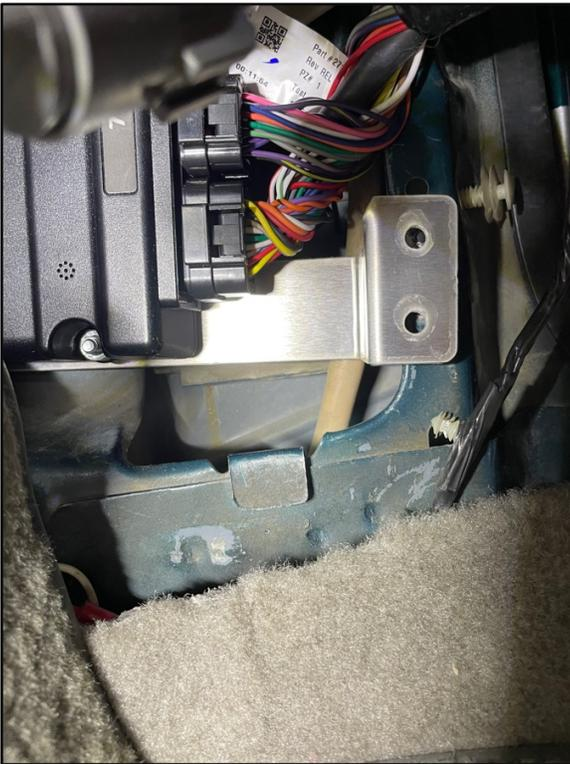
Bolt the Terminator ECU to the bracket as shown.
