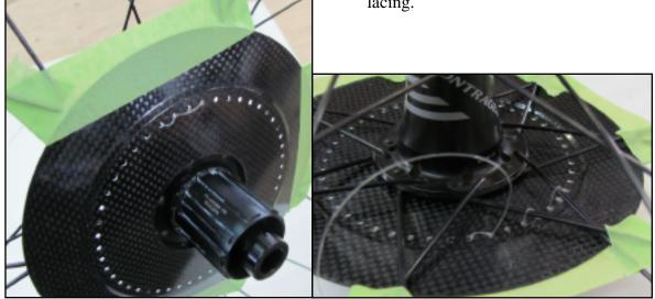
**Step 3 -** Start lacing with the long end of line. Go through a hole in the disc that is next to a spoke. Go around the spoke and back through the next hole so there is a tight loop around the spoke as shown.
