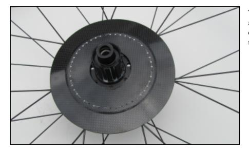
The finished product laced up to a wheel and ready to keep your chain from jamming between the spokes and cassette.
