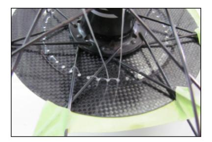
**Step 3 -** Continue lacing around the disc. Depending on your spoke pattern you may skip a hole in order to go through the disc next to a spoke. It is important that you come through the disc next to a spoke, around the spoke and then back through the next hole in the disc. Pull the line snug after going through each hole.
