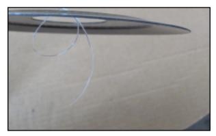
**Step 1 -** Loop the lacing line through two holes in the disc as shown. Leave a long tail on the wheel side to tie later.
