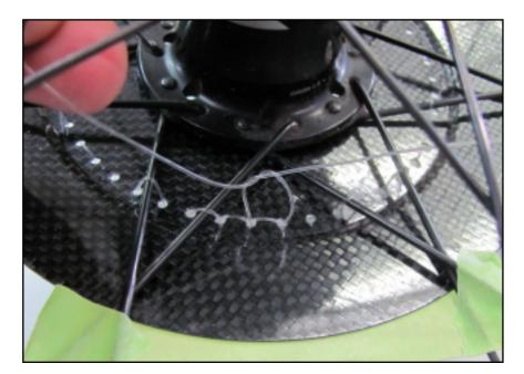
**Step 4 -** Once you have laced around the disc, finish with the same loop you started. You should have two ends side by side as shown. Tie the ends together with a simple overhand knot, pull tight and add a second knot on top.
