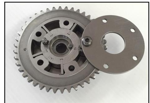
3. The lockouts are precision machined to fit in one section better than the rest. The lockout should be installed into the void that has the tightest fit. Push the lockout block fully down into the phaser. Our blocks have been designed to fit snug and there can be a large variance in phasers. If the block is too tight you can file down the top 'pointy' edge to fit. It doesn't take much to make a big difference in fit. Note the locks for Dormans do not require filing.
