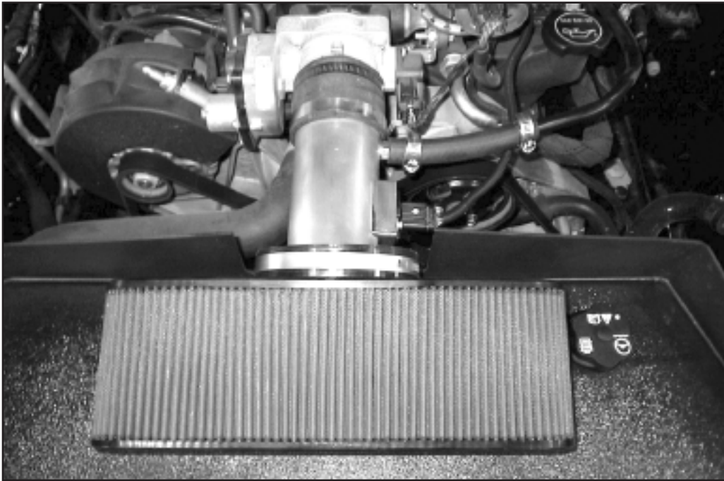
The finished install showing front mounted filter and mass air meter, ram air box as well as the relocated coolant overflow tank.
